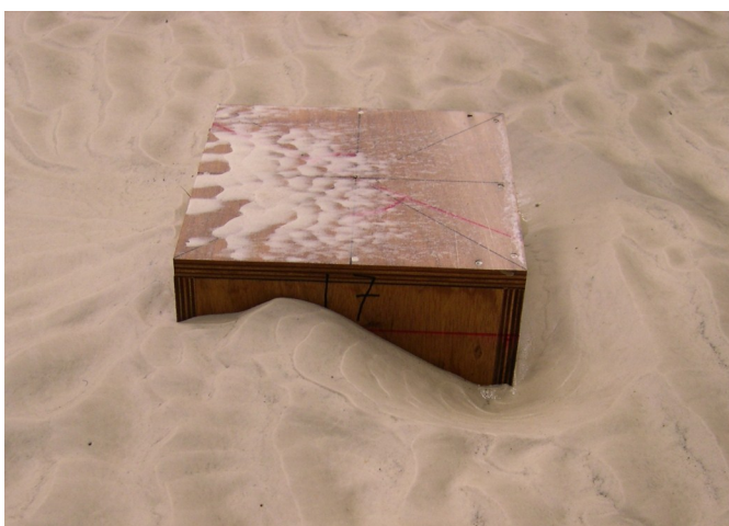
Example of scour around a box shaped structure representative of a gravity based structure.
